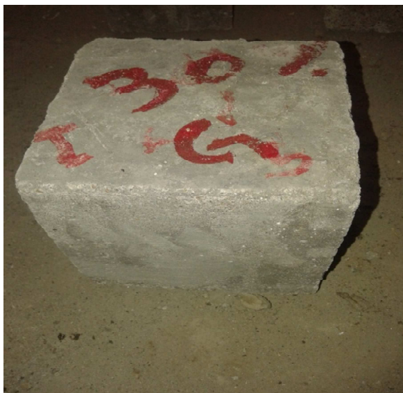
Figure 10: conventional concrete after submersed in acid-water bath
