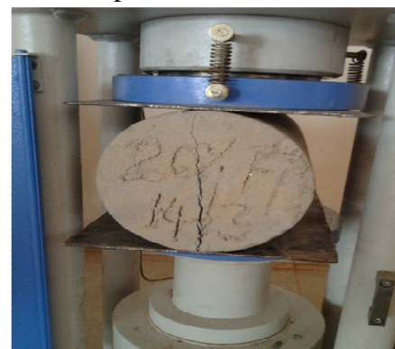
Figure 5: cylinder failure under tensile loading
