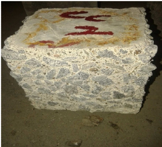
Figure 10: conventional concrete after submersed in acid-water bath
