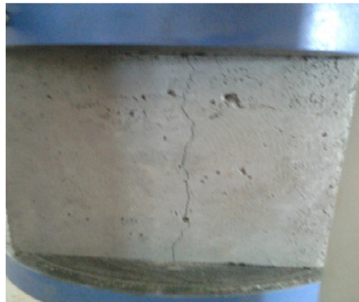
Figure 1 : Cube specimen failure under compressive load
