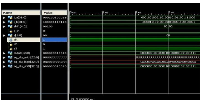
Fig-8: Simulated Waveform for Shift Unit
