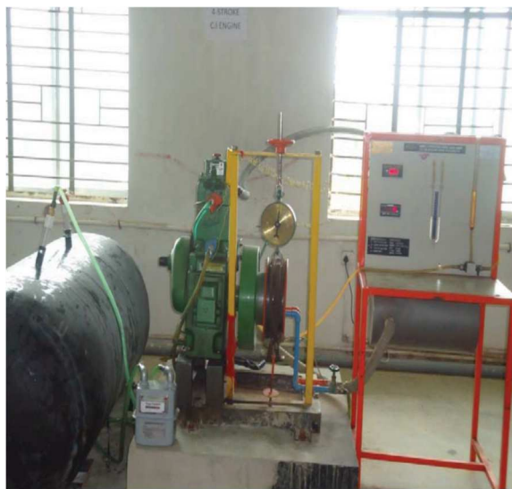
Fig.3 Experimental setup of biogas-fuelled C.I engine
