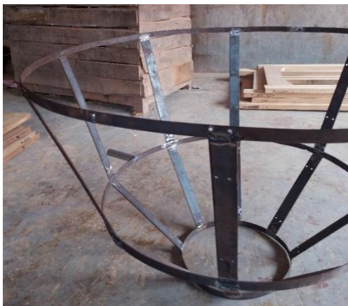
Figure 9. Fabricated dish frame
