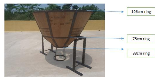
Figure 1. Side view of the DAES solar cooker
