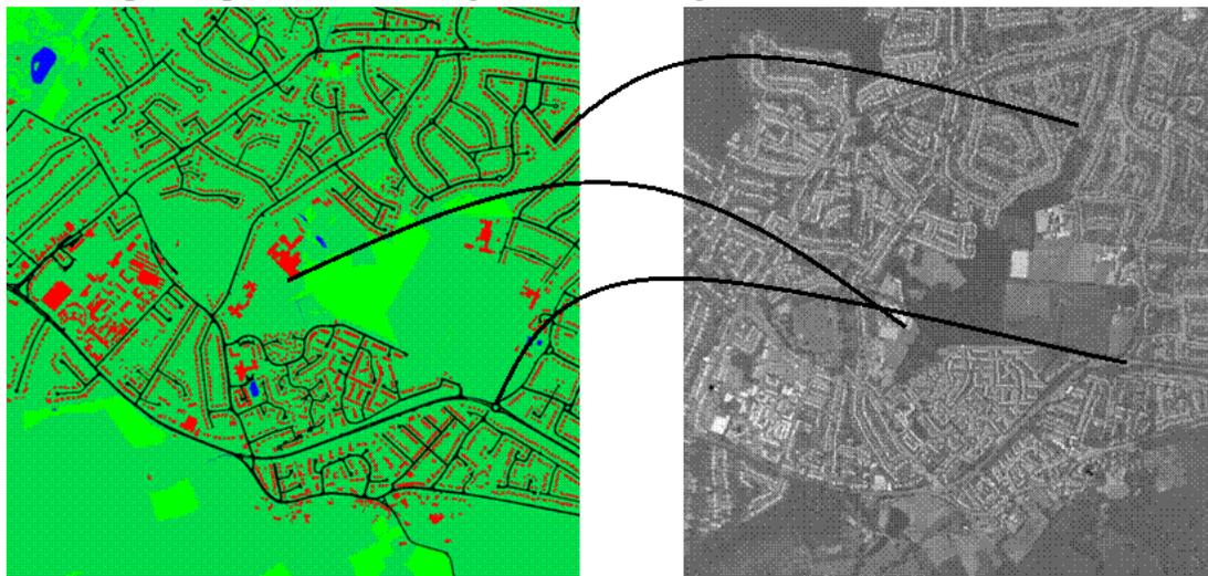
An illustration of the use of ground control points from verification data (left) to geo-correct image data (right)
