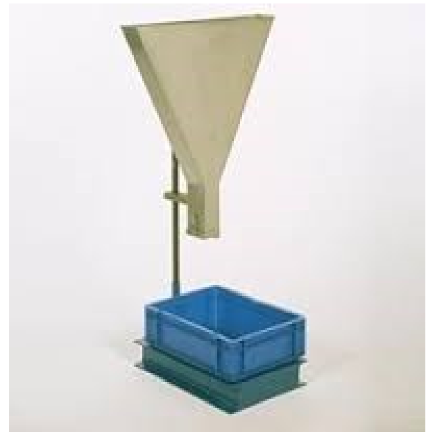
Figure 4.6 V- funnel test
