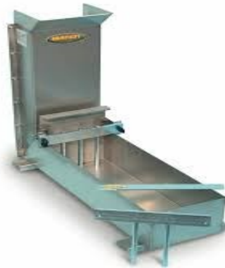
Figure 4.4 L-box test Table 4.2 L - box test results
