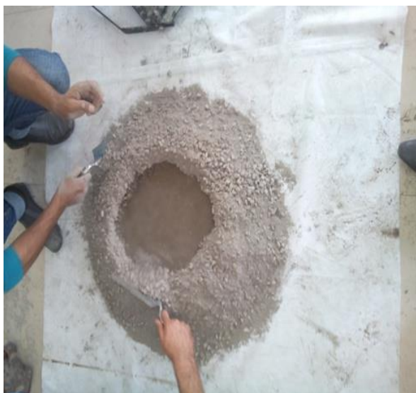
Figure 3-Mixing of Fibres into Concrete
