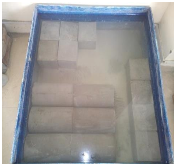
Figure 4-Curing of Concrete Blocks
