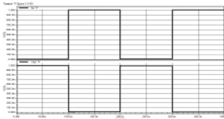
Figure 10: Input and output waveform of NOT gate using GDI method in 150nm technology
