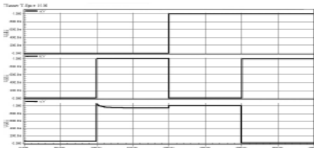
Figure 4: Input and output waveform of a XOR gate using GDI method in 150nm technology
