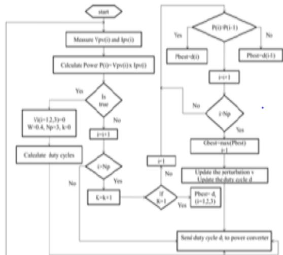
**Fig 4. Flow chart of modified PSO technique.**
