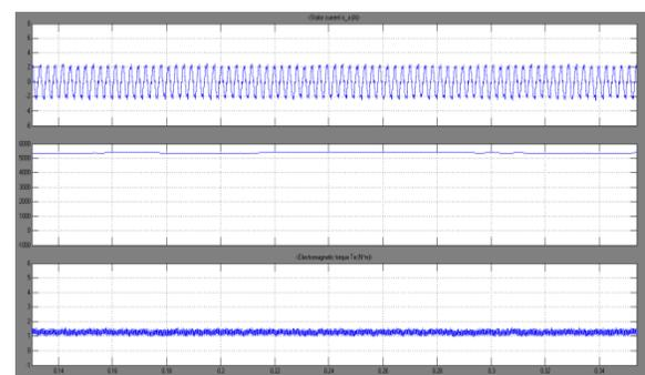
Fig 28.Simulation wave form of stator current, speed and electromagnetic torque
