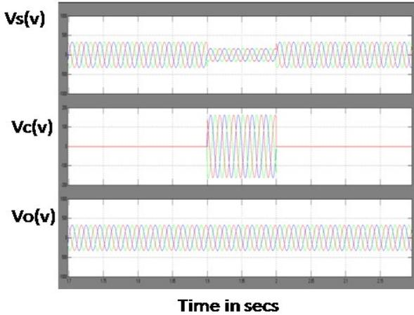
Fig 11 Simulated output wave form of Source voltage, Compensating Voltage and Load Voltage with UPQC.
