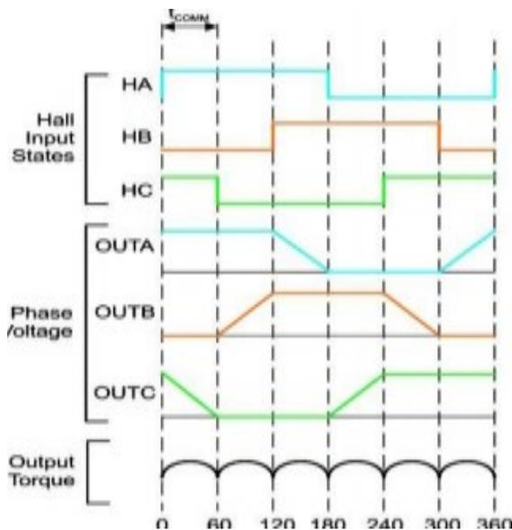
**Fig 5 Hall signals & Stator voltages**
