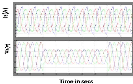
Fig 7 simulation wave form of Source current and Source voltage without UPQC.
