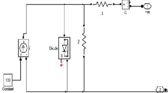
**Fig.19. Simulink circuit of Photo Voltaic Cell for UPQC**
