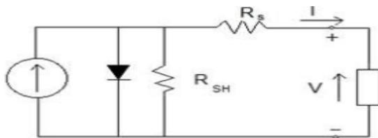
**Fig. 2. Electrical Equivalent Circuit Model of PV Cell**
