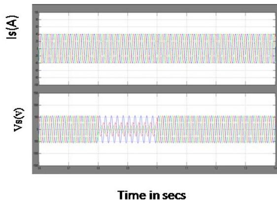
Fig 25 simulation wave form source current and voltage when BLDC load connected.
