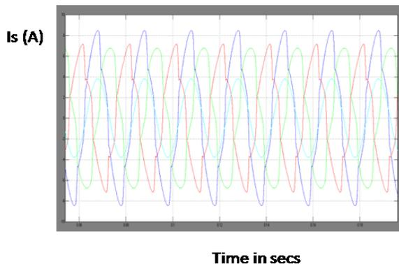
Fig. 8 Simulated wave form of the load current for RL load.
