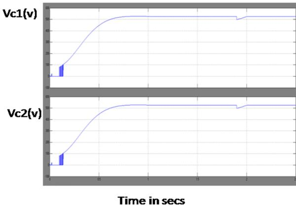
Fig. 12. Simulated output wave form of the Voltage across C1 and C2 capacitors.
