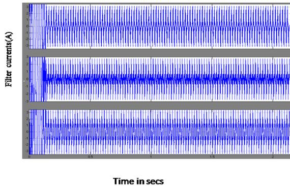
**Fig. 17. Simulated output wave form of the filterside currents not changing**
