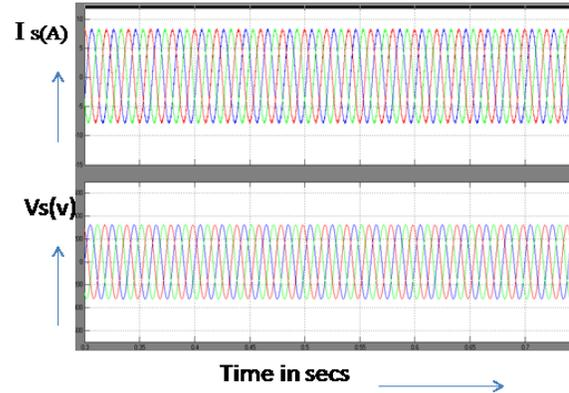
**Fig 20 simulation wave form of Source voltage and current UPQC PV systems**
