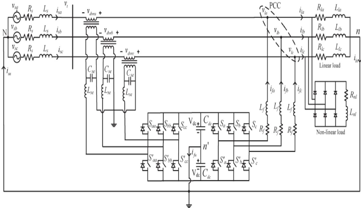
Fig.1. Equivalent circuit of neutral-clamped VSI topology-based UPQC
