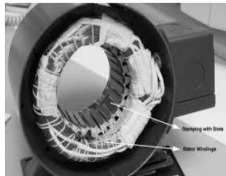
**Fig 3 BLDC motor stator construction**
