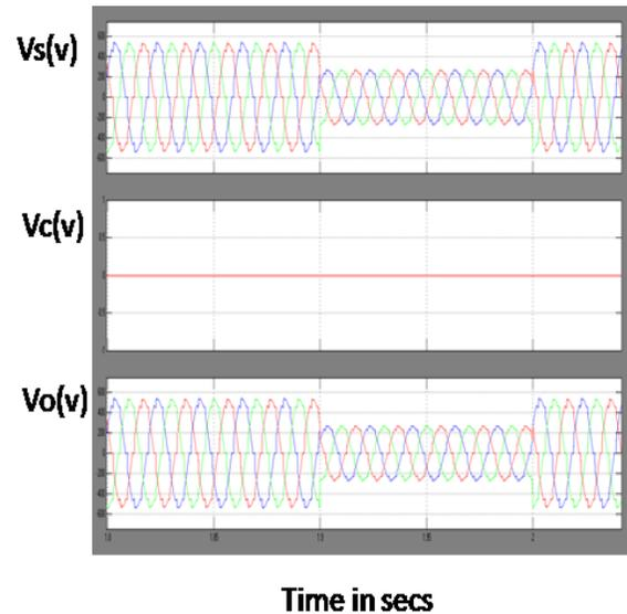
Fig.9 Simulated output wave form of Source voltage, Compensating voltage and Load voltage without UPQC.
