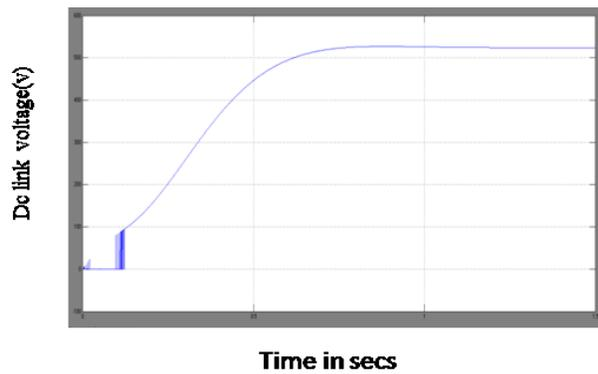
Fig 24 simulation wave form dc-link voltage for BLDC motor controller.
