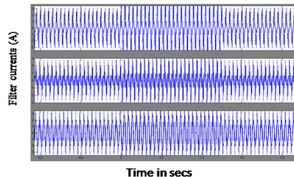
**Fig. 22. Simulated output wave form filter currents changing to reduce variations of source currents.**
