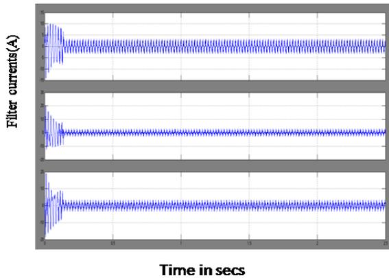
Fig. 13. Simulated output wave form of the filterside currents with UPQC
