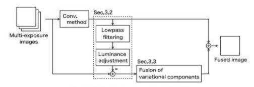
Fig. 1: Block diagram of proposed method.
