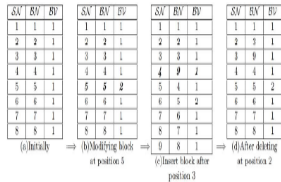
Fig. 2. Changes in the MVT due to different dynamic operations on copies of a file F = \{b_j\} | 1 \leq j \leq 8 .
