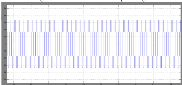
Fig 5 simulation wave form of input line voltage at 500v
