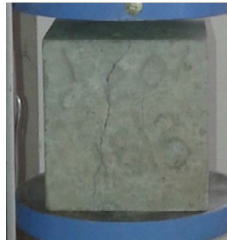
Figure 1: Cube specimen failure under compressive load
