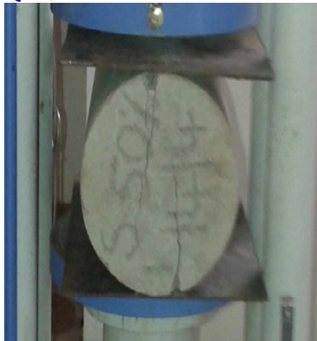
Figure 3: Cylinder failure under tensile loading
