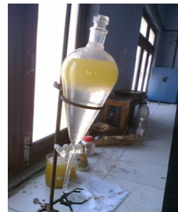
Figure-4.6 Separation of water and biodiesel after Water washing of biodiesel
