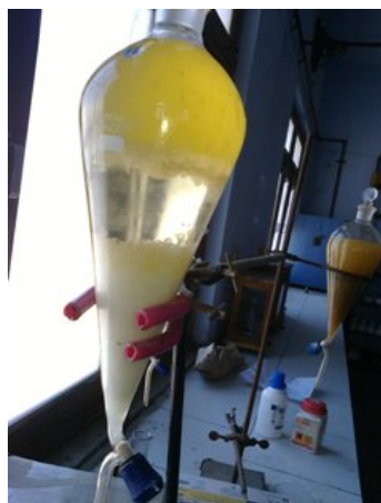
Figure-4.5 Separation of biodiesel from glycerol and excess methanol
