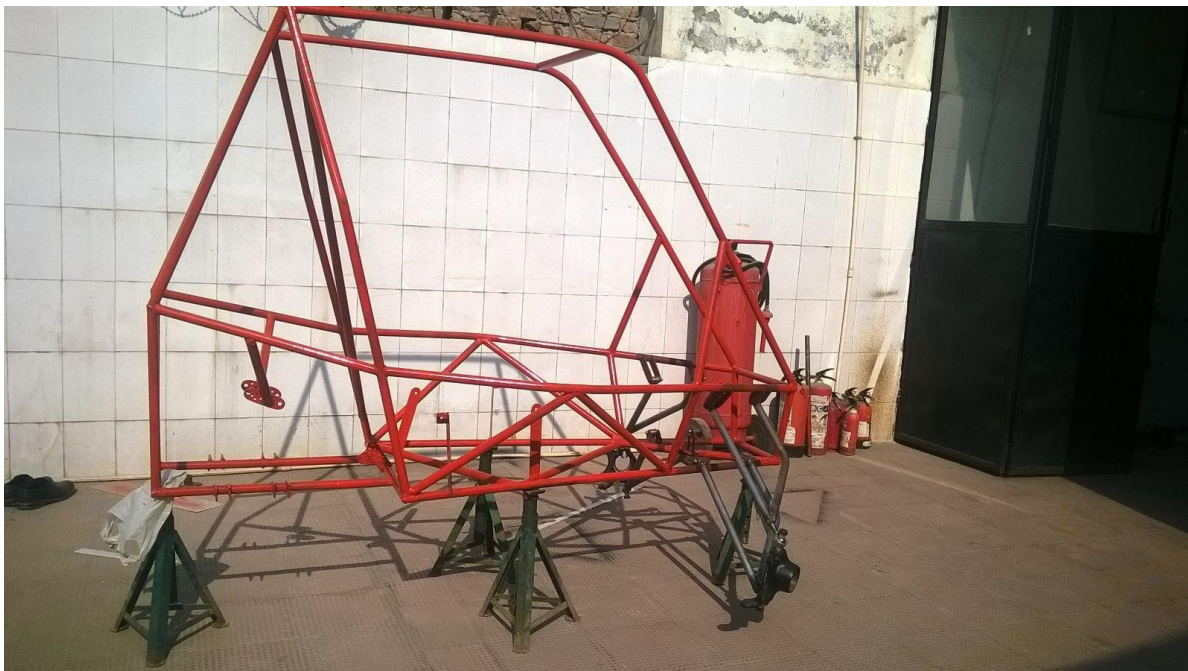
Fig. 25: Complete painted chassis
