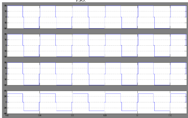
Fig.9. Individual H-bridge voltage and seven level inverter output voltage with PSO.
