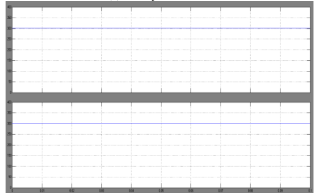
Fig.11. simulation waveform of proposed system input voltage with flying capacitor.
