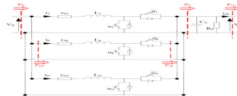
Fig. 1. N parallel boost converters structure with one output capacitor.
