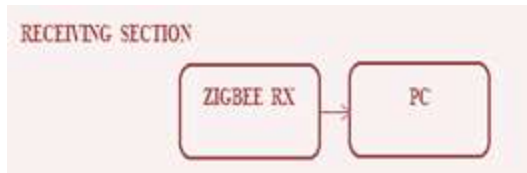
Fig.2 Block diagram of fault indicator using ZigBee protocol
