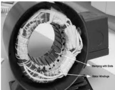
Fig.3. BLDC motor stator construction
