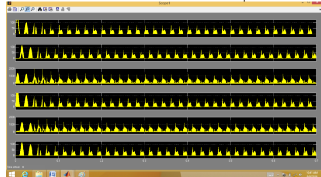
Fig 9 simulation waveform of inductor current, switch voltage and current of Buck-Boost converter.
