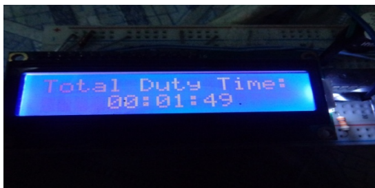
Figure 12. Stopping of pump with Indication of total
