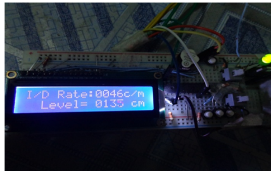
Figure 8. starting of pump with Indication of water level condition
