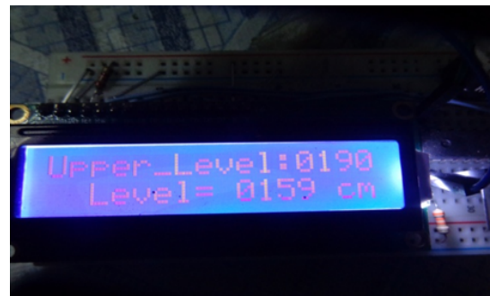
Figure 6. Setting upper level of water
