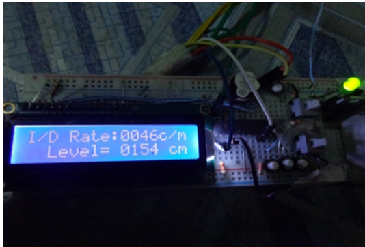
Figure 9. starting of pump with Indication of water level
