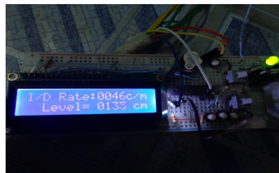
Figure 8. starting of pump with Indication of water level condition
