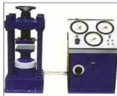
Figure ; Compression test Equipment
