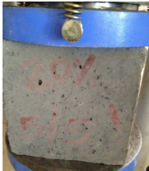
Figure 2.0 Cube Specimen Failure under Compressive Load
