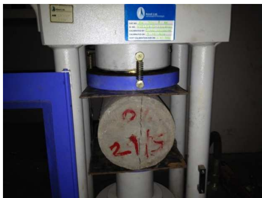
Figure 4.0 Cylinder Failure under Tensile Loading
