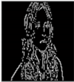
Fig. 2c Edge Detection by Improved Canny Algorithm
