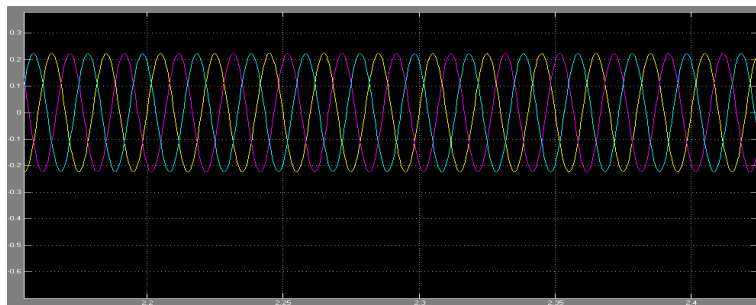
Fig 4. Three-phase grid-side currents in the grid-connected PV inverters
