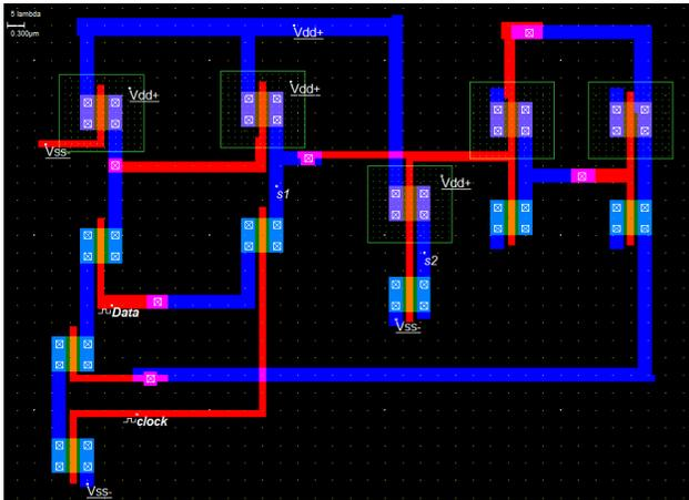
Figure 7. Layout of the proposed Flipflop
