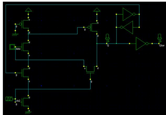
Figure 5. Schematic of the proposed flipflop.
