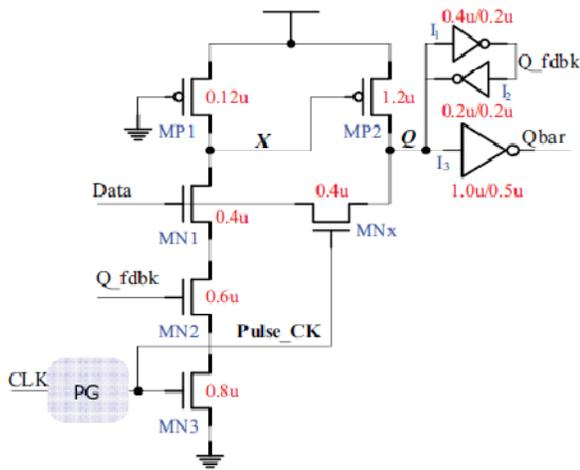
Figure 4. Schematic of the proposed P-FF design.
