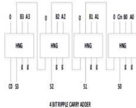
Fig3:4 Bit Ripple Carry Adder
