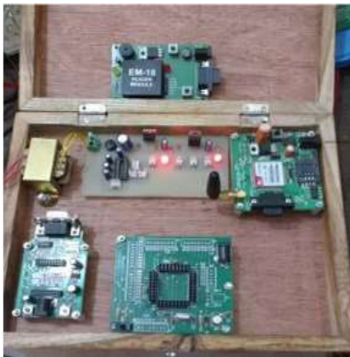
Fig: 2. Prototype of intelligent traffic control system, ambulance clearance and stolen vehicle detection
