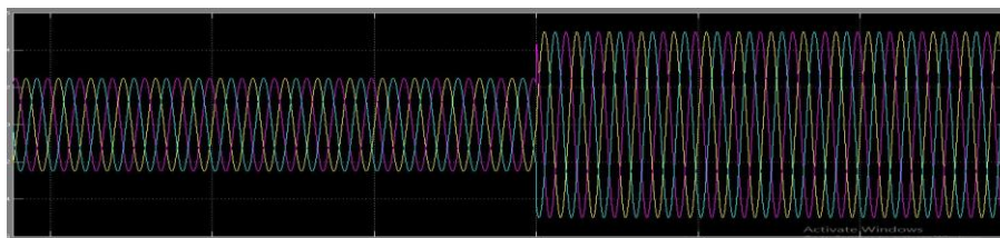
Fig 17. Output current of the dc/ac VSI
