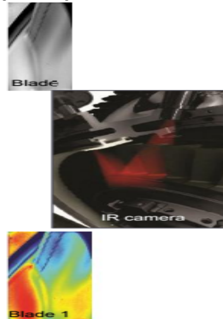
Figure 4: Compressor turbine blade temperature measurement
