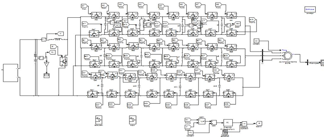
**FIG: Three-phase power schematic of the proposed seventeen-level inverter configuration formed by cascading three-level flying capacitor inverter with three H-bridges using a single dc link.**
