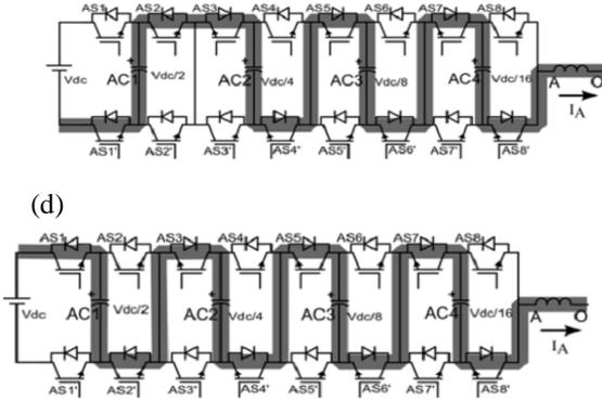
(d) Fig. 3. Switching Redundancies for pole voltage of  $V_{dc}/16$ . (a) Current path for switching state (0, 0, 0, 0, 0, 0, 0, 1). (b) Current path for switching state (0, 0, 0, 0, 0, 1, 1, 0). (c) Current path for switching state (0, 0, 0, 1, 1, 0, 1, 0). (d) Current path for switching state (0, 1, 1, 0, 1, 0, 1, 0). (e) Current path for switching state (1, 0, 1, 0, 1, 0, 1, 0).
