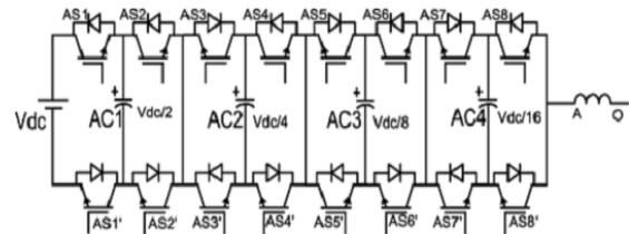
Fig. 2. One phase of the proposed 17-level inverter configuration formed by cascading three-level flying capacitor inverter with three H-bridges using a single dc link.
