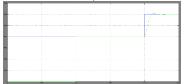
Fig 17 Simulation waveform for Dynamic performance of the proposed closed loop power control
