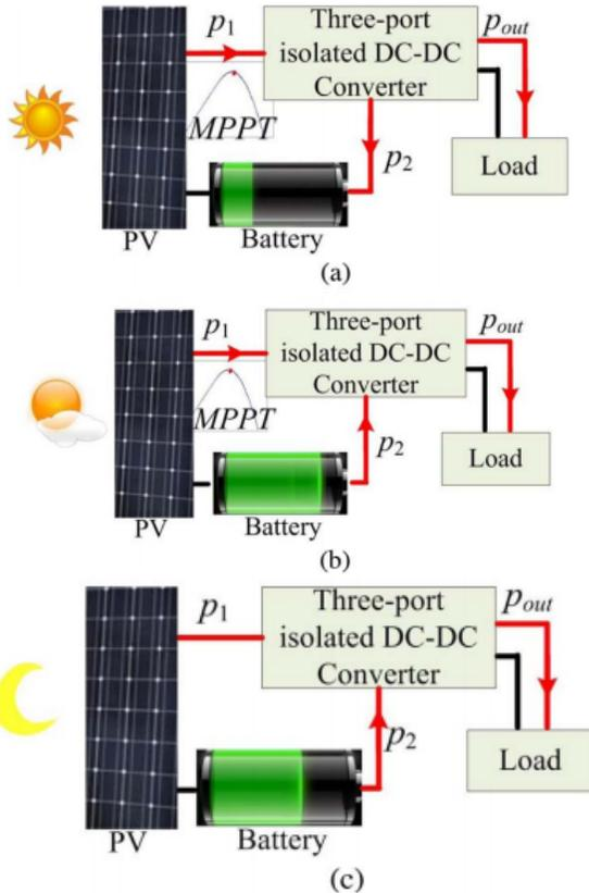
Fig.5. Three working scenarios of the converter (the arrows show the directions of energy flow). (a) Scenario 1 ( $p_1 > p_{out}$ ): PV works in MPPT mode and the battery works in charge mode to absorb the surplus solar energy. (b) Scenario 2 ( $p_1 < p_{out}$ ): PV works in MPPT mode and battery works in discharge mode to provide the deficient energy. (c) Scenario 3 ( $p_1 = 0$ ): there is no solar energy available and battery is discharged to supply load.
