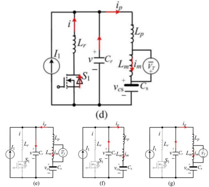
Fig. 4. Equivalent circuits for different operating modes. (a) Mode 1:  $S_1$  is on,  $i > 0$ , and  $v_p = V_T$ . (b) Mode 2:  $S_1$  is on,  $i > 0$ , and  $i_p = i_m$ . (c) Mode 3:  $S_1$  is on,  $i > 0$ , and  $v_p = -V_T$ . (d) Mode 4:  $S_1$  is being turned off,  $i < 0$ , and  $v_p = -V_T$ . (e) Mode 5:  $S_1$  is off,  $i = 0$ ,  $v_p = -V_T$ . (f) Mode 6:  $S_1$  is off,  $i = 0$ , and  $i_p = i_m$ . (g) Mode 7:  $S_1$  is off,  $i = 0$ , and  $v_p = V_T$ .
