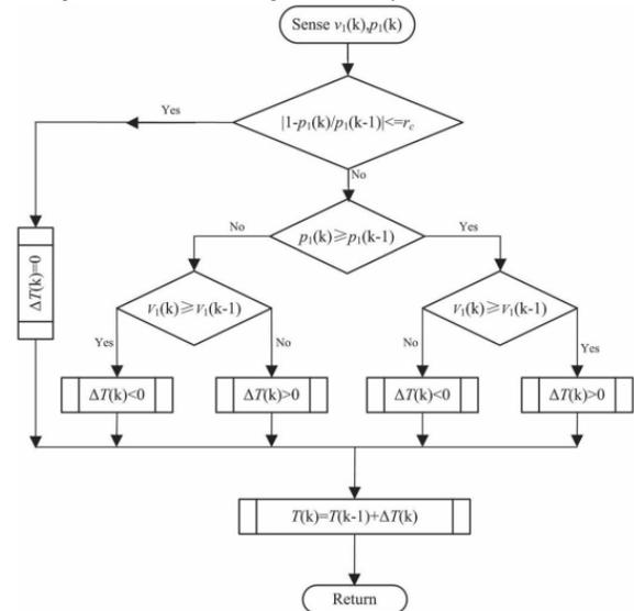
Fig.7. Flowchart of the MPPT algorithm.
