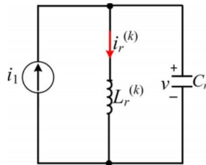
Fig.2. Equivalent resonant circuit.
