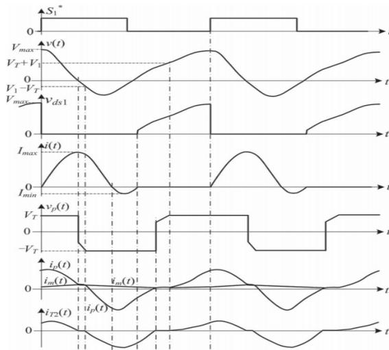
Fig.3. Steady-state waveforms of the proposed converter.
