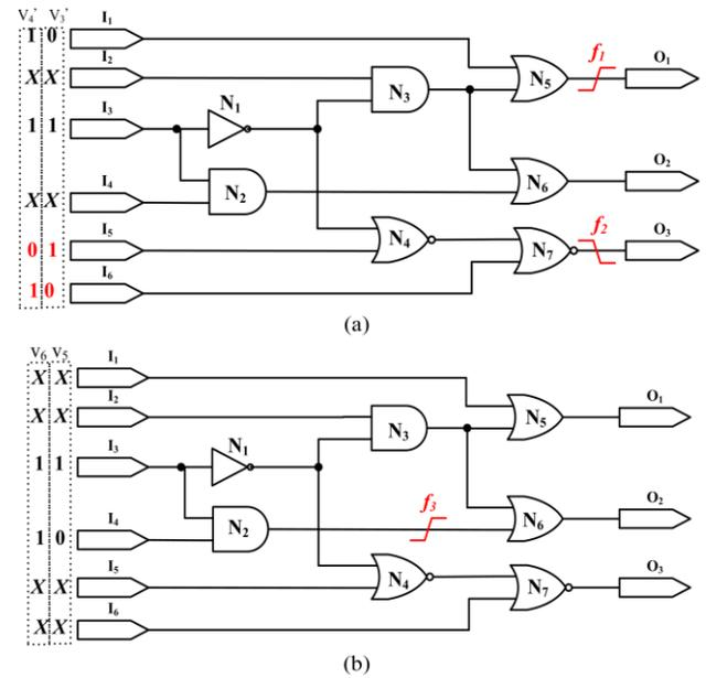
Fig:3. Two new pattern pairs detect the faults  $f_1$  (N5 slow-to-rise),  $f_2$  (N7slow-to-fall), and  $f_3$  (N2 slow-to-rise). (a) Refined P2 that detects  $f_1$  and  $f_2$ . (b) New pattern pair P3 that detects  $f_3$ .
