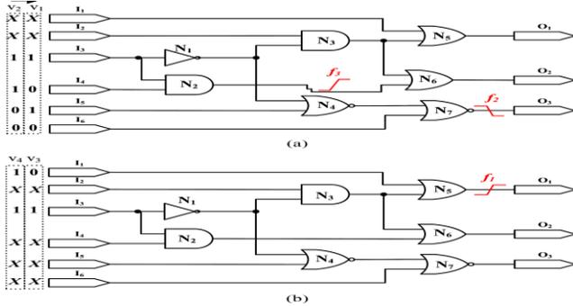
Fig2. Example of two partially-specified pattern pairs in the original ATPG test set to detect the faults  $f_1$  (N5 slow-to-rise),  $f_2$  (N7 slow-to-fall) and  $f_3$  (N2 slow-to-rise). (a) Partially-specified pattern pair P1 detects  $f_2$  and  $f_3$ . (b) Partially-specified pattern pair P2 detects  $f_1$ .
