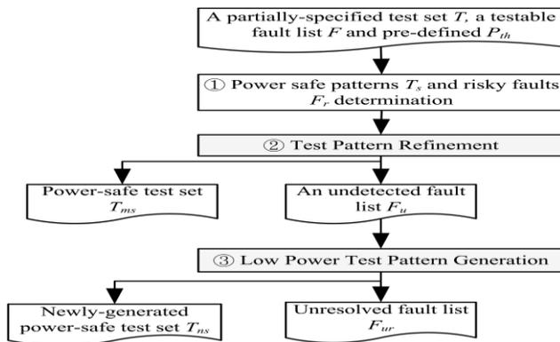
Fig.4. Overview of proposed capture-power-safe test pattern determination procedure.
