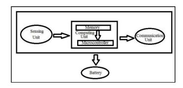
Sensing Unit- It consists of the sensor deployed at the node which collects data at the ground level. This data is the physical raw data which is sampled and converted to the
