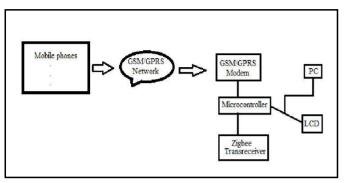
In the Ground Section, the Zigbee Transceiver receives the information and sends to the ARM controller. The LCD connected to the controller displays the information in the Ground Section. The controller is connected to the GSM modem through RS232.A number of mobile phones to which the data has to be sent is connected to the modem through GSM network. In addition the controller is connected to PC; the measured values are continuously displayed and stored in the PC for future use.
