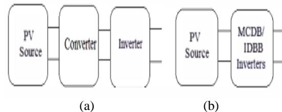
Fig 5 MPPT control methods (a) indirect method (b) direct method
