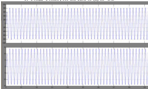
Fig 22 Output voltage and current of inverter and current of inductance, when the inverter connected to the load,  $R=50n, L=50mH$ , for the case of (b)  $m=0.7$
