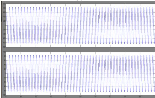
Fig 20 Output voltage and current of inverter and current of inductance, when the inverter connected to the load,  $R=1\Omega$ , for the case of (a)  $m=0.7$
