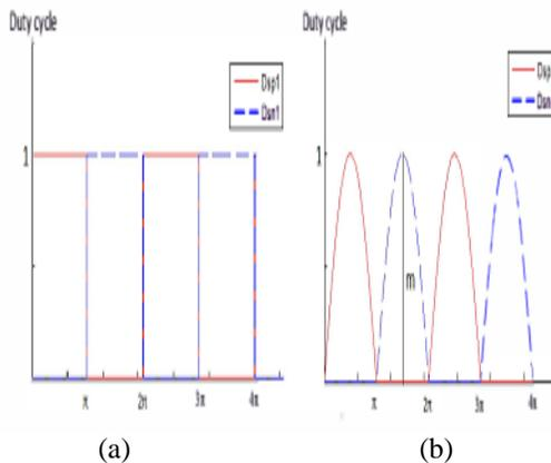
Fig.3.3 switching signals of the switches of proposed MCDB inverter (a) switches  $S_{pi}$  and  $S_{ni}$  (b) switches  $S_p$  and  $S_n$
