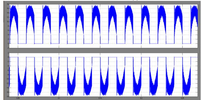
Fig 9 Current waveform of inductance  $L_p$  and  $L''$  when the inverter connected to the load of  $R = 1\Omega$ , for the case of  $m = 0.3$
