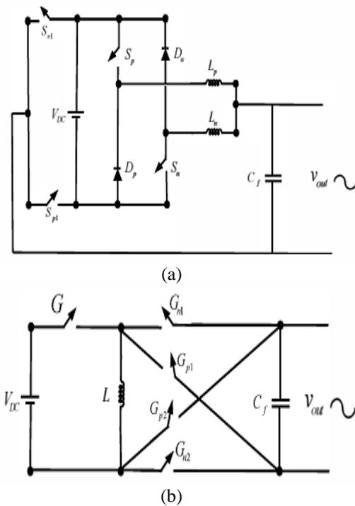
Fig 1 proposed (a) MCDB (b) IDBB, inverters
