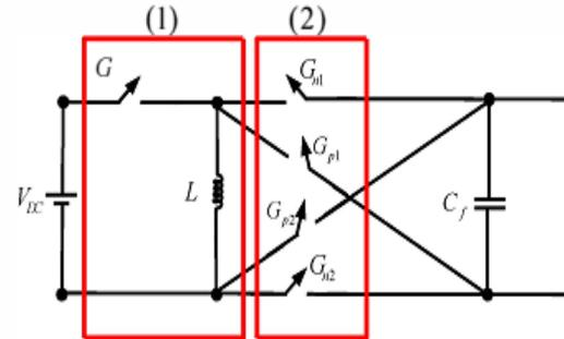
Fig 4 Structure of proposed IDBB inverter
