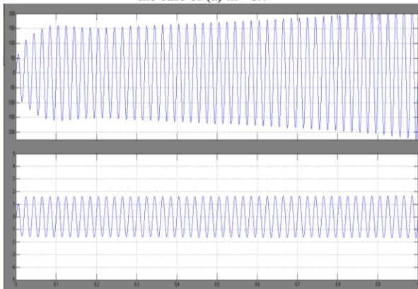
Fig 21 Output voltage and current of inverter and current of inductance, when the inverter connected to the load,  $R=50n, L=50mH$ , for the case of (a)  $m=0.3$
