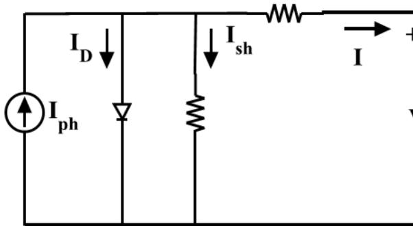
Fig 6 Equivalent circuit of Single diode modal of a solar cell
