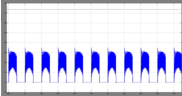
Fig 11 Current waveform of inductance  $L_p$  and  $L''$  when the inverter connected to the load of  $R = 1\ \Omega$ , for the case of  $m = 0.7$
