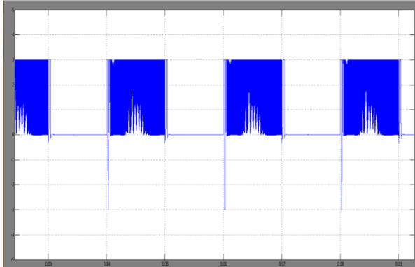
Fig 13 Current waveform of inductance  $L_p$  and  $L''$  when the inverter connected to the load of  $R = 50\ \Omega, L = 50\ \text{mH}$ , for the case of (a)  $m = 0.3$
