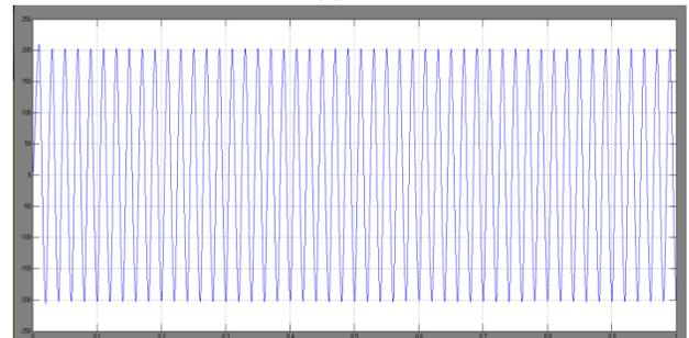
Fig 10 Output voltage of inverter after inductance and output voltage of inverter before inductance, when the inverter connected to the load,  $R = 1\Omega$ , for the case of  $m = 0.7$
