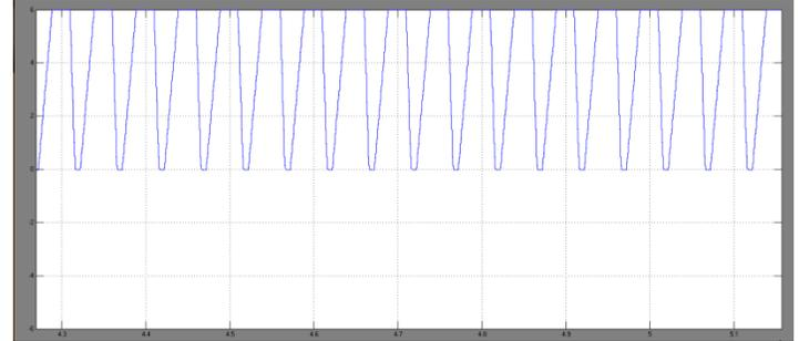
Fig 15 Current waveform of inductance  $L_p$  and  $L''$  when the inverter connected to the load of  $R = 50\ \Omega, L = 50\ \text{mH}$ , for the case of (a)  $m = 0.7$
