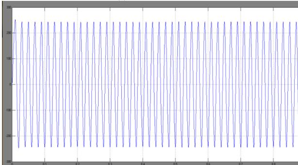
Fig 14 Output voltage of inverter after inductance and output voltage of inverter before inductance, when the inverter connected to the load of  $R=50\ \Omega, L=50\ \text{mH}$ , for the case of (a)  $m=0.7$
