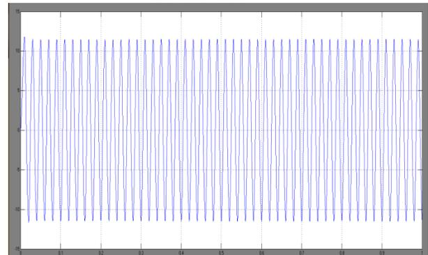
Fig 17 simulation wave form of output voltage with PV
