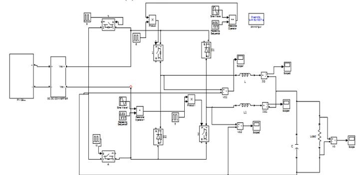
Fig 16 Matlab/simulation circuit of Modified Cascaded Dual Buck converter with PV
