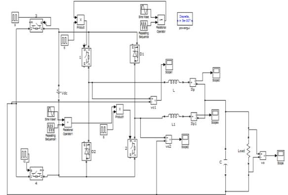
Fig 7 Matlab/simulation circuit of Modified Cascade Dual Buck converter
