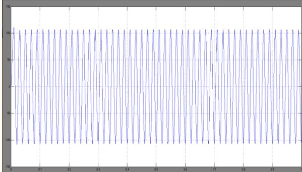
Fig 12 Output voltage of inverter after inductance and output voltage of inverter before inductance, when the inverter connected to the load of  $R=50\ \Omega, L=50\ \text{mH}$ , for the case of (a)  $m=0.3$
