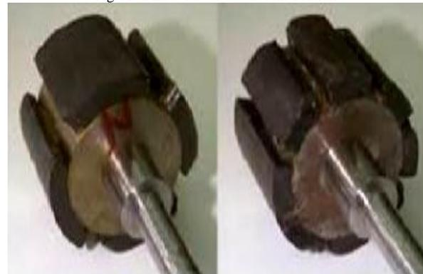
Fig.12. BLDC motor Rotor construction.
