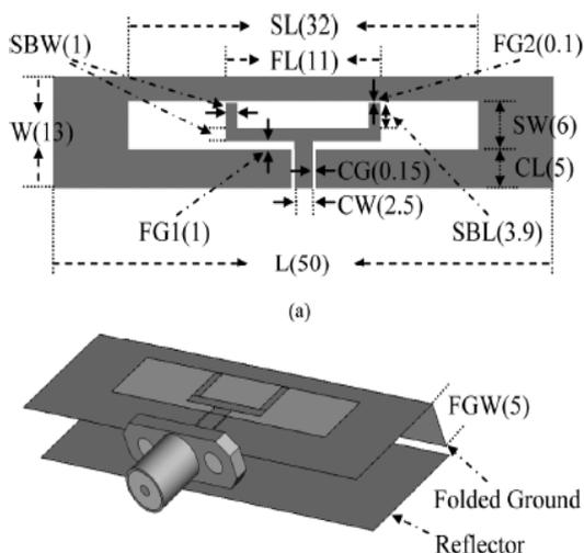
*Fig. 1. Structure of the RWSA and its major dimensions (unit in millimeter): (a) the antenna element; and (b) the entire configuration, comprising the reflector and the extended folded ground (detailed parameter descriptions are listed in Table I).*
