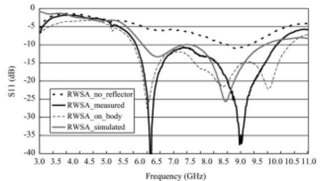
Fig. 4. Measured and simulated reflection coefficients of an RWSA.
