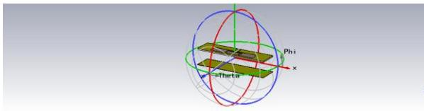
Fig. 2. Impedance bandwidth enhanced by introducing a reflector and a folded ground.
