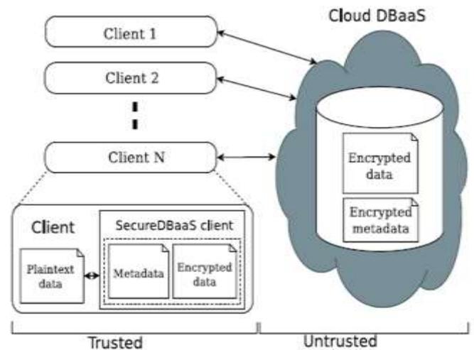
Fig 1: Architecture of Untrusted secure Encrypted Cloud Database
