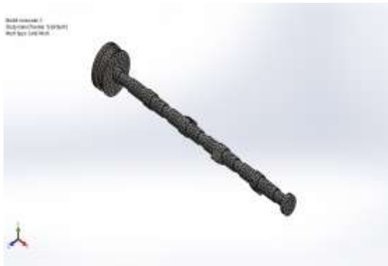
Figure 11: Meshed model of camshaft
