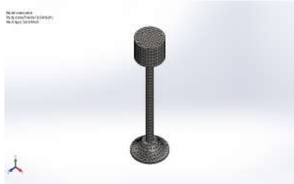
Figure 8: Meshed model of valve
