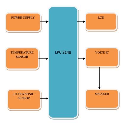
Different types of ultrasonic sensor and fire sensors are available in the market. Ultrasonic sensor measures the round trip delay which is directly proportional to output pulse width of the distance measured. The block diagram of proposed hardware is shown in Fig.1.The microcontroller triggers the ultrasonic sensor and receives echo when it detects any obstacle. The microcontroller collects information from ultrasonic sensor (and fire sensor if any fire is detected) and computes the distance.
