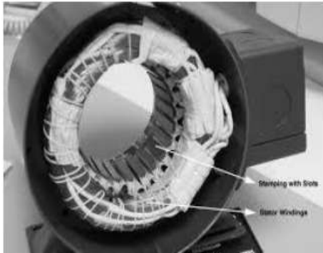
Fig.4. BLDC motor stator construction
