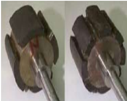
Fig.5. BLDC motor Rotor construction.
