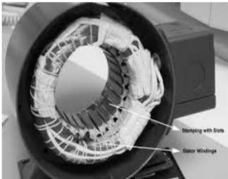
Fig.3. BLDC motor stator construction
