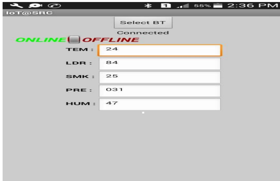
Fig 5: monitoring in android application installed in mobile
