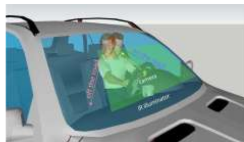
Figure 1: Eyes off the road (EOR) detection system.
