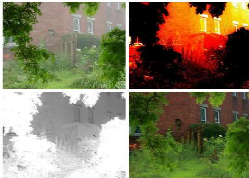
Fig.1. An overview of the proposed dehazing method. Top-left: Input hazy image. Top-right: Restored depth map. Bottom-left: Restored transmission map. Bottom-right: Dehazed image.
