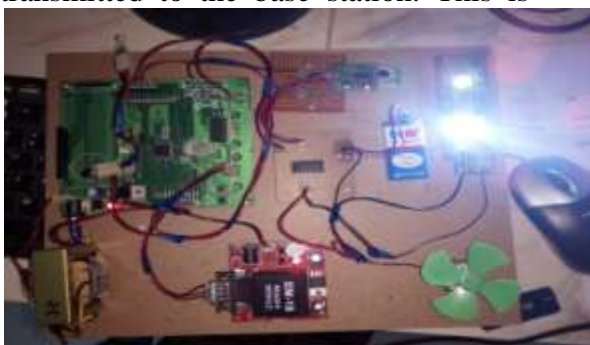
Fig30: if intensity low lights on automatically
